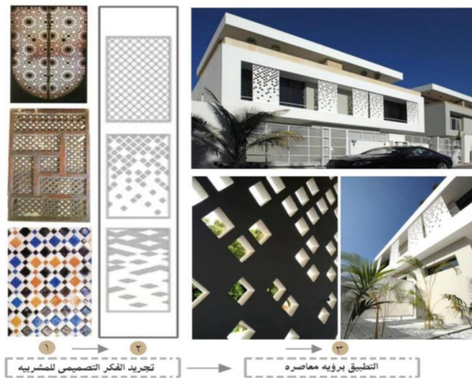
Fig (7) integration between modern technology and traditional intellect to design a bay (mashrabiya) The source (Kamel, Ahmed Samir, Gamal, Dina Fekry)
